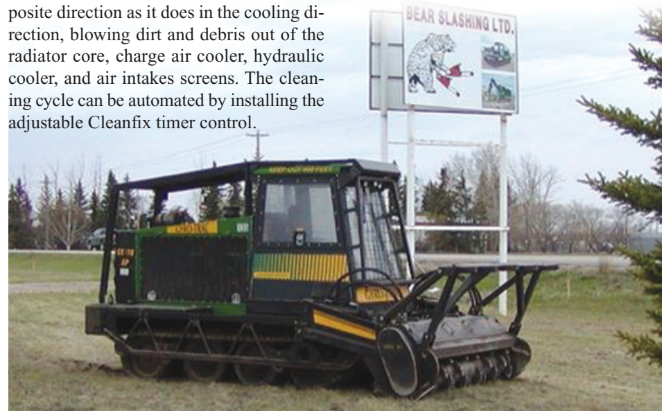
Another leading supplier of heavy equipment to Bear Slashing is Gyro-Trac, shown above. Bear Slashing purchased the first machine built by Gyro-Trac and currently has 13 of the machines. Gyro-Trac manufactures mulchers with a patented captive track system and mulching cutter-heads.
